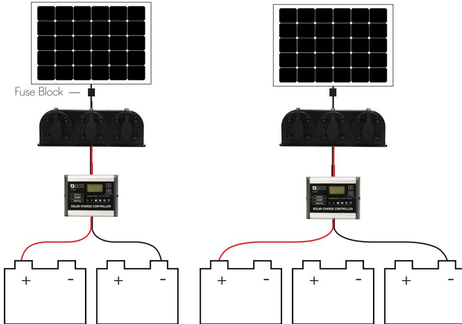
How **NOT** to wire a solar controller for 2 batteries
