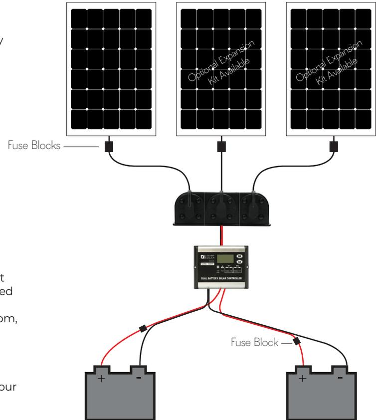
When wiring a solar kit to multiple batteries, it is important to remember that your batteries are wired together. To gain the most from your solar kit, be sure to place the positive wire on the first battery in the sequence and the negative wire on the last battery in the sequence. This is true regardless of the number of batteries in the bank.
