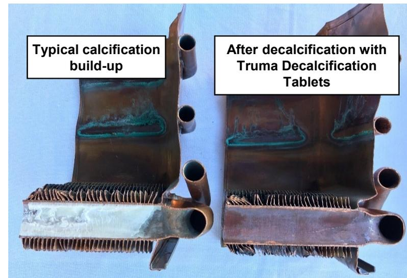
An integrated water consumption meter recognizes (after hot water consumption of approx. 1585 gallons/ 6000 liters) that decalcification is necessary. The assumed water hardness is “hard” and cannot be changed. The yellow status LED 3 on the control panel indicates that decalcification is necessary (goes off briefly about every seven seconds).
